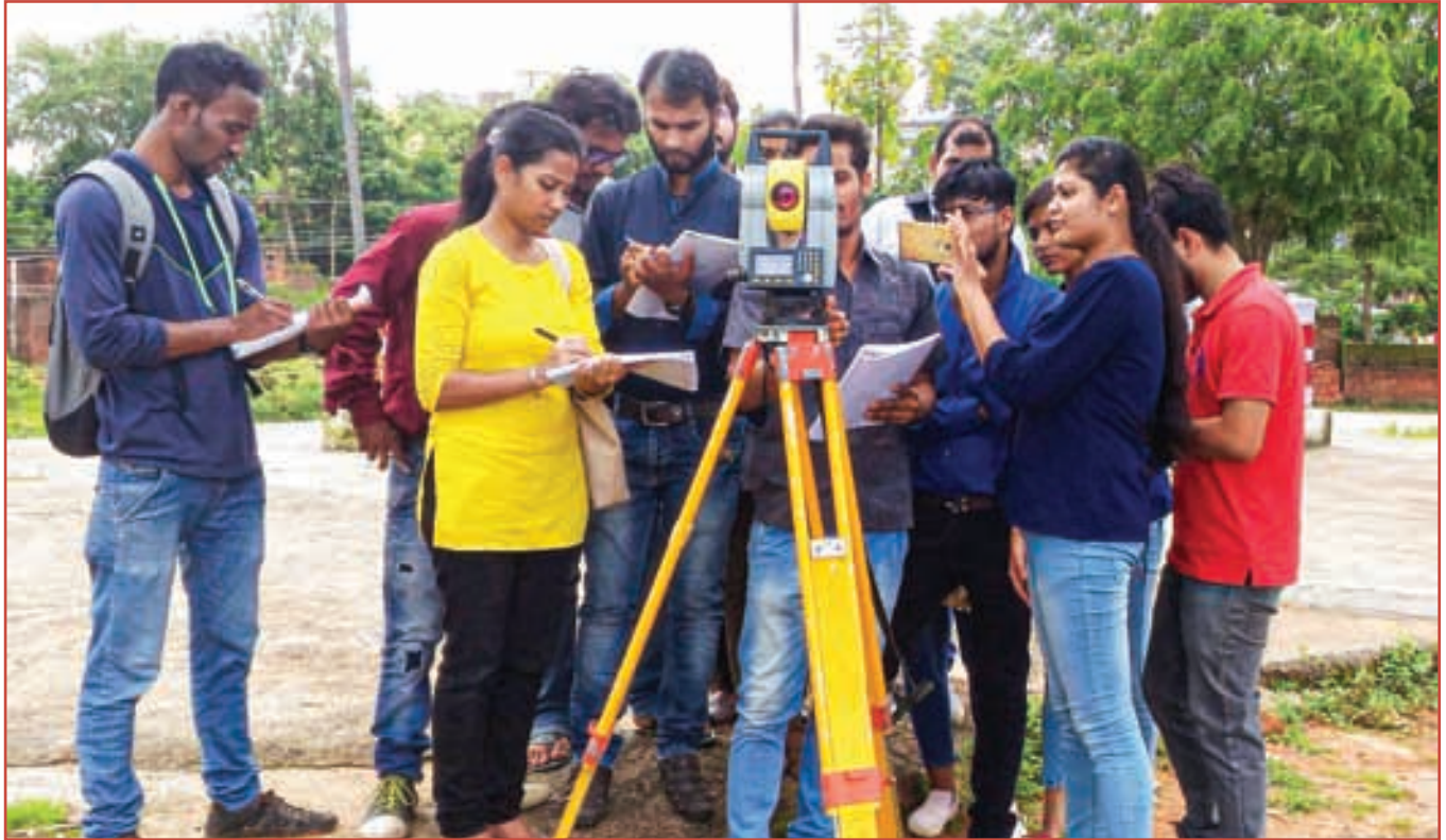
Field Practical on Electronic Total Station (ETS) near Jogo Hills, Ranchi
